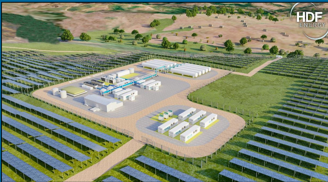
FIGURE 3. CONCEPT IMAGE OF THE HDF SOLAR PV FARM AND THE HYDROGEN GENERATION, STORAGE, AND FUEL CELL FACILITIES. 29
