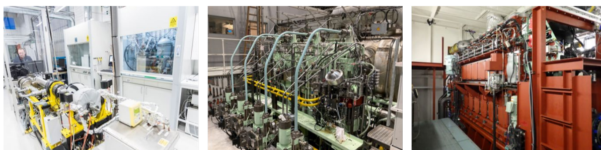
FIGURE 22. SOME AMMONIA ENGINES ARE IN DEVELOPMENT. IMAGES COURTESY OF THE MANUFACTURERS (WARTSILA, MAN ENERGY SOLUTIONS, AND IHI POWER SYSTEMS).
